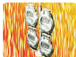
08、模壳焙烧 Mold Preheat
