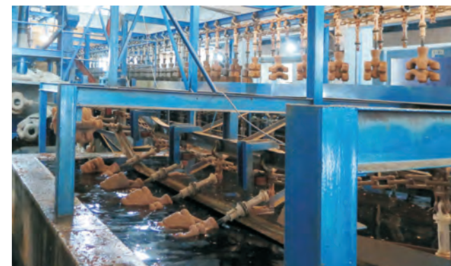
自动淋砂 Automated Stuccoing
